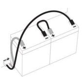
**2.** Attach battery cables to battery as shown in illustration above "Battery connection".
