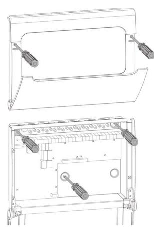
Mount the panel, using pre drilled screw positions, to the wall. This will prevent any possible brick dust contamination of the panel internal circuitry. Use Three No.10 x 1  $\frac{1}{4}$ " (5.0 x 30mm approx.) pan head screws. When using 20mm conduit entry direct to ensure a wide distribution of pressure when tightening the coupling.
