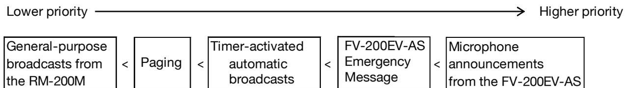
Example: If the microphone announcements from the FV-200EV-AS is in progress, only that broadcast will be performed, and other broadcasts will not be made.
