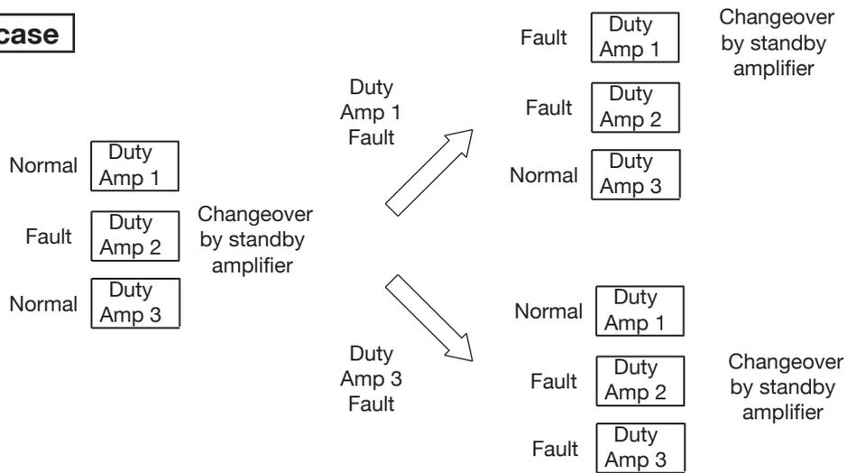
FV-200CA-AS have 7 LED fault indicator for connected amplifier including standby amplifier fault and have 6 LED changeover indicator. Only one LED changeover indicator can light at once, but LED fault indicator will light as many as fault occur at duty or standby amplifier.
