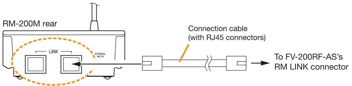
Without AC adapter plugged into RM-200M power will be supplied from system Power Supply through FV-200RF-AS DC Supply terminal.
