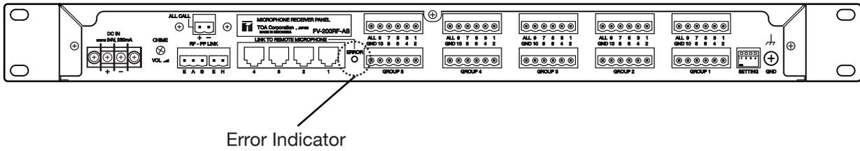
A communication failure has occurred between the RM-200M and the FV-200RF-AS. The previous status is automatically restored if communications return to normal.
