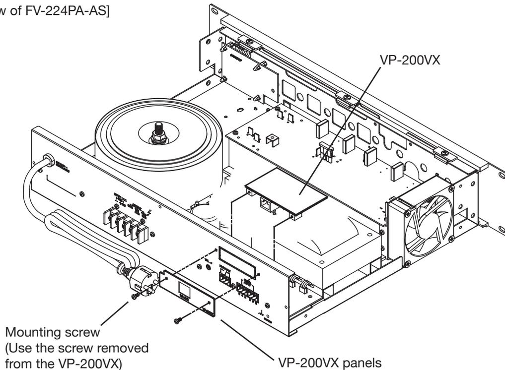
Step 5. Plug the VP-200VX's connector into the connector on the circuit board inside the amplifier.
