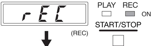
When recording starts, the Recording indicator lights and the "rEC" (REC) indication appears for about 1 second on the Status display, followed by the "EMER" (EMER) indication.
