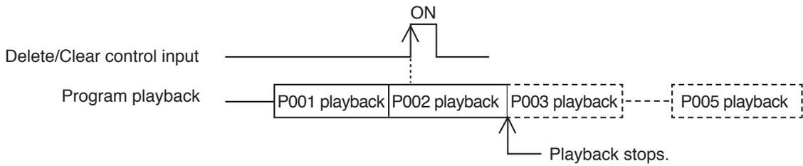
In the example above, playback stops when P002 playback is complete and no subsequent programs are played.
