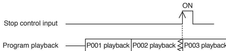
In the example above, P002 playback is interrupted, then the subsequent Program P003 playback will start.
