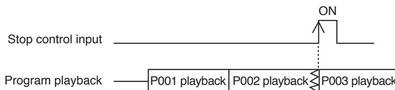
In the example above, P002 playback is interrupted, then the subsequent Program P003 playback will start.
