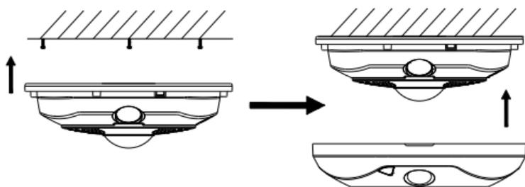
Figure 2-3 Install the Camera
