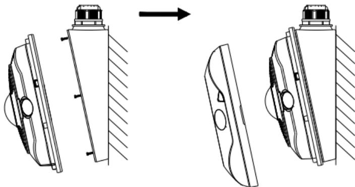
Figure 2-7 Install the Camera Body and Cover
