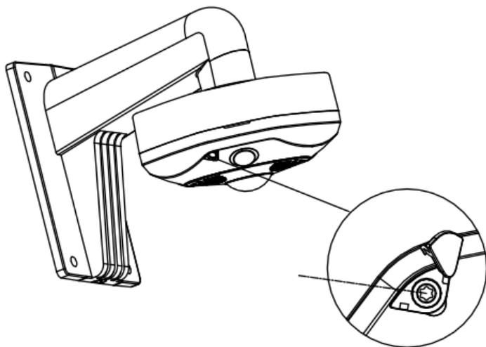
Figure 2-14 Tighten the Screw on the Camera Cover
