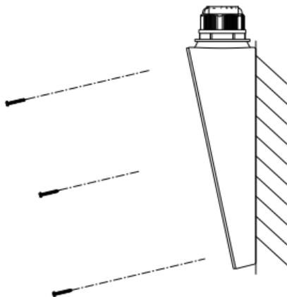
Figure 2-6 Hammer the Screws
