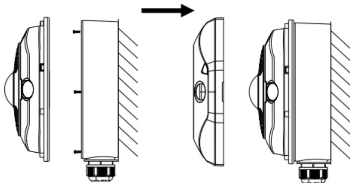
Figure 2-10 Install the Camera Body and Cover
