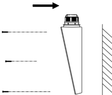
Figure 2-5 Fix the Slant Mounting Base
