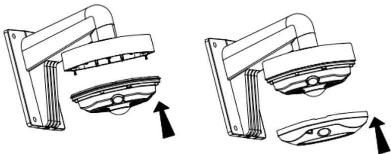
Figure 2-13 Install the Camera Body and Cover
