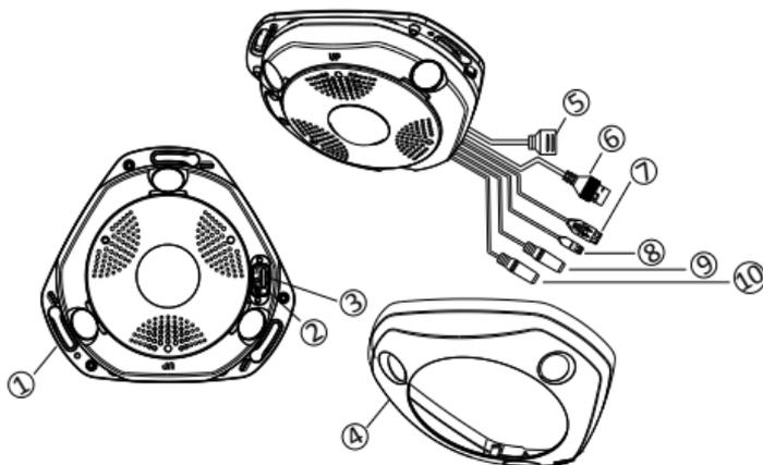
Figure 1-2 Disassemble of Fisheye Camera
