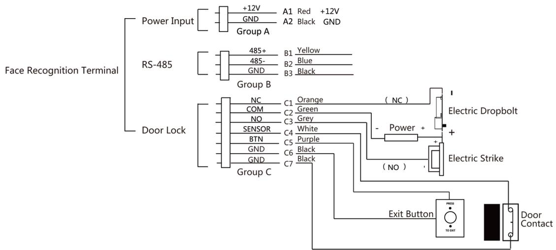
**Figure 4-2 Device Wiring**
