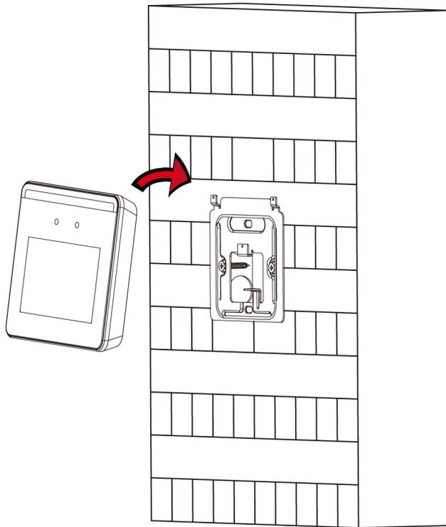
**Figure 3-5 Install Device**
