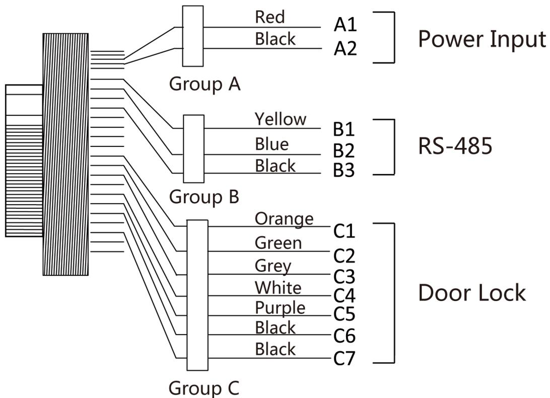
**Figure 4-1 Terminal Diagram**
