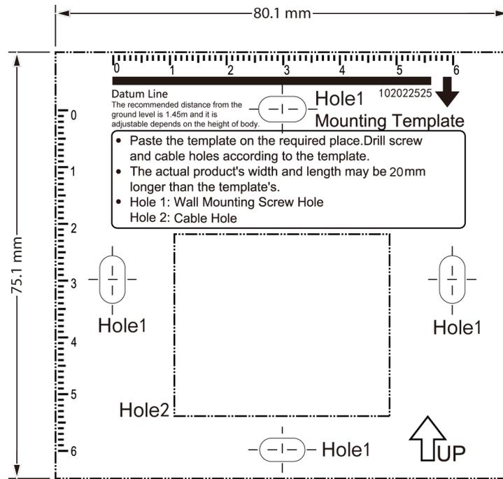
**Figure 3-2 Mounting Template**
