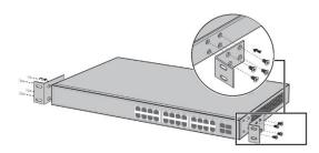
Put PoE switch on the appropriate location of the rack, crutch by bracket; using the L-shaped bracket to fix the two sides of rack with screw, make sure PoE switch is installed on the rack smooth and steady.
