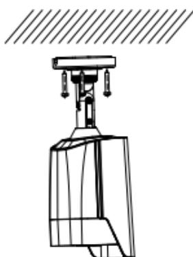
Figure 2-9 Fix the Camera to the Ceiling
