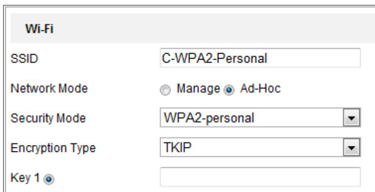
The screenshot shows the same 'Wi-Fi' settings panel as Figure 4-2, but with the 'Ad-Hoc' radio button selected under 'Network Mode'. All other settings, including 'SSID', 'Security Mode', 'Encryption Type', and 'Key 1', remain the same.
